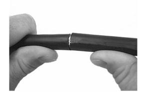
Figure 11 – Flex the cable to separate the inner cable jacket.
