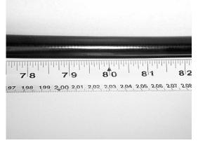
Figure 1 - Measure and mark the section of cable jacket to be removed.
