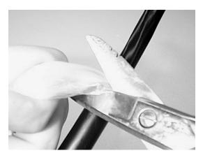
Figure 28 – Cut the dielectric strength members as required.
