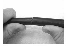
Figure 22 – Separate the cable jacket.
