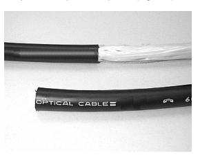
Figure 5 - Remove the 5-inch section of outer jacket.
