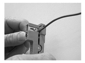
Figure 18 – Ring cut the buffer tubes with a buffer tube removal tool.
