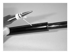
Figure 7 - Pull the rip cord through the outer jacket.
