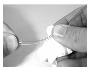
Figure 19 - Clean the fibers with isopropyl alcohol.
