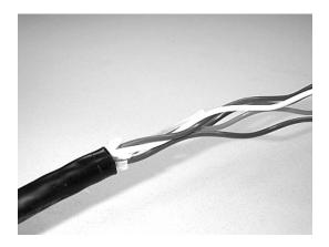
Figure 17 - Unwrap the buffer tubes.
