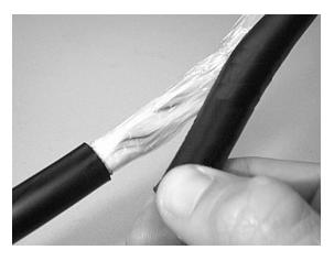
Figure 8 - Remove the outer cable jacket.
