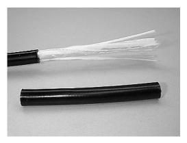
Figure 13 - Remove the 5-inch section of inner jacket.
